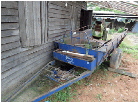
<Corroded farming machine stored in place without the ceiling - Kha Young village>
