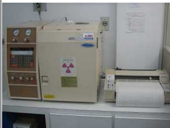
Gas chromatograph provided by Japan’s ODA in 1994 to the Evandro Chagas Institute, one of the implementing organizations of “Project for Strengthening of the Health Vigilance System on Methylmercury in Tapajos River Basin, Amazon” (Technical Cooperation)
