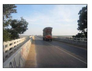
contributing substantially to the axle load problem and premature deterioration of road pavements. The photo shows the traditional Bedford two-axle truck that is assembled in Pakistan.
