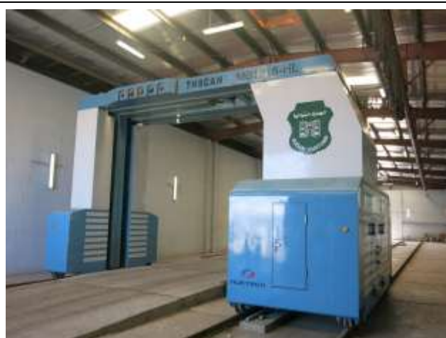
One of two scanners, Port Sudan. (NucTech, 6Mev, double-tunnel).
