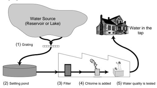
The figure above shows how water supplied to houses in cities is made fit for drinking.
