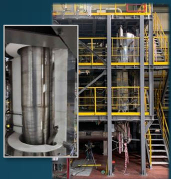
Fluidized Bed Reactor 50 kg/batch
